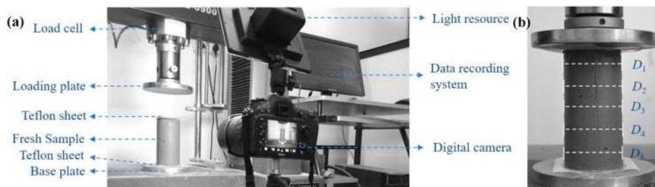
Fig. 5. (a) Setup for the unconfined uniaxial compression test and (b) photograph of a fresh specimen during image analysis.
