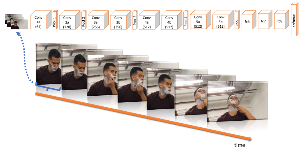
Figure 3. This figure shows the deep learning model OAD-3D-CNN, which is used for the monitoring of the daily-life activities of the users. Our model has 8 3D convolutions, 5 max-pooling layers and 3 fully connected layers, followed by a softmax output layer. All 3D convolution kernels are 3 \times 3 \times 3 with stride = 1 in both spatial and temporal dimensions. Note that in each box we indicate the number of filters. The 3D pooling layers are denoted pool1 to pool5, where the pooling kernels are 2 \times 2 \times 2 , except pool1, for which it is 1 \times 2 \times 2 . The fully connected layers have 4096 output units.
