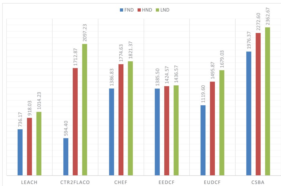
Figure 12. FND, HND and LND for 150 nodes in a 100 m × 100 m area with BS at (50, 50) m.
