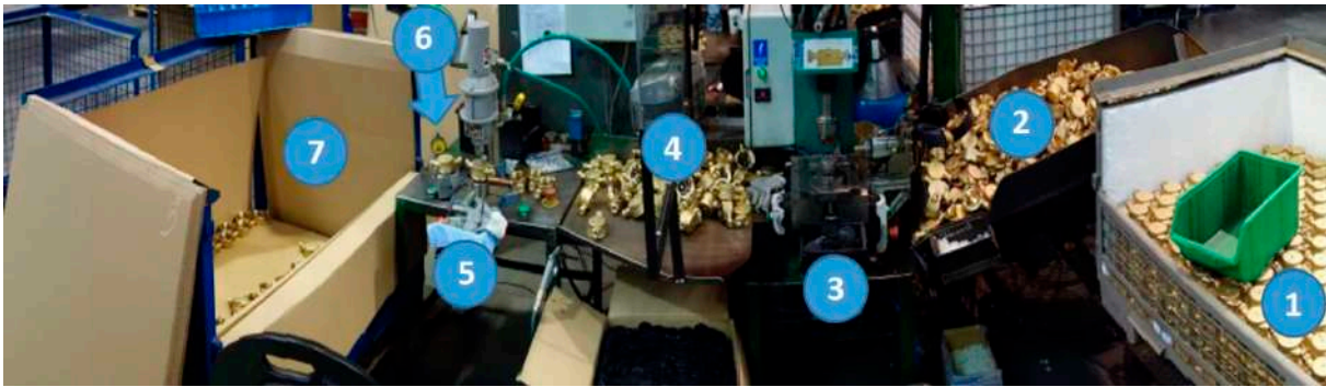
Figure 2. Assembly line for water meter bodies with elements: 1—Storage bay with a basket of processed water meter bodies intended for assembly components, 2—Auxiliary tray for machined bodies, 3—Station for assembling the strainer and damming plate in the water meter body, 4—Transitional storage bay for partially assembled bodies, 5—Station for mounting the axle in the water meter body, 6—Control of the depth of the axle seating in the water meter body, 7—Storage bay with a basket for the assembled water meter bodies.
