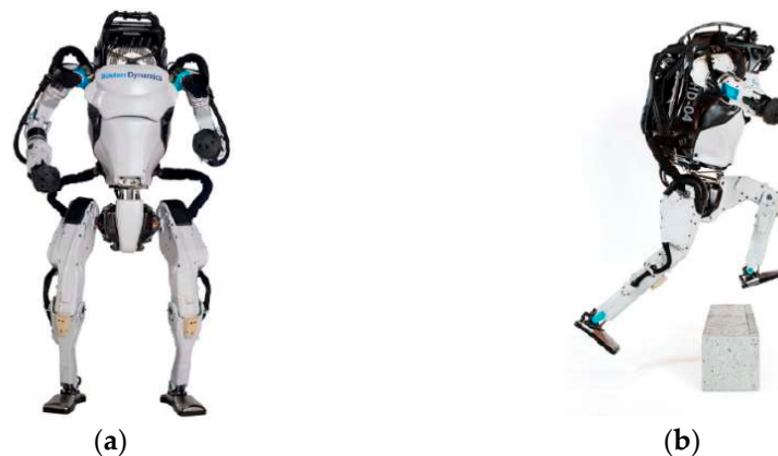
Figure 7. Atlas: (a) overall look, (b) jumping over an obstacle [55].
