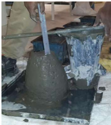
Figure 2. Slump test of fresh concrete mixtures containing different proportion of heavyweight fine aggregate using cone mold.
