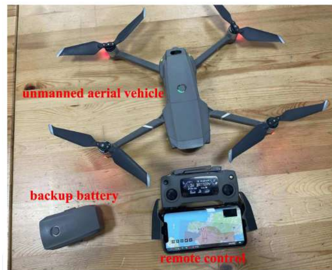
Figure 11. Physical diagram of Mavic 2 DJI's unmanned aerial vehicle.
