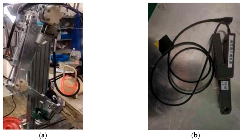
Figure 28. Moment-following test: (a) The exoskeleton; (b) Current clamp.
