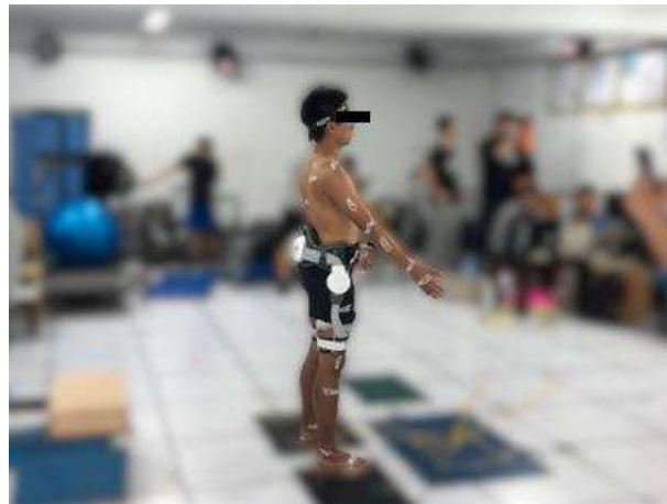
Figure 21. A subject wore the robotic exoskeleton with EMG sensors and reflectors attached to his body.
