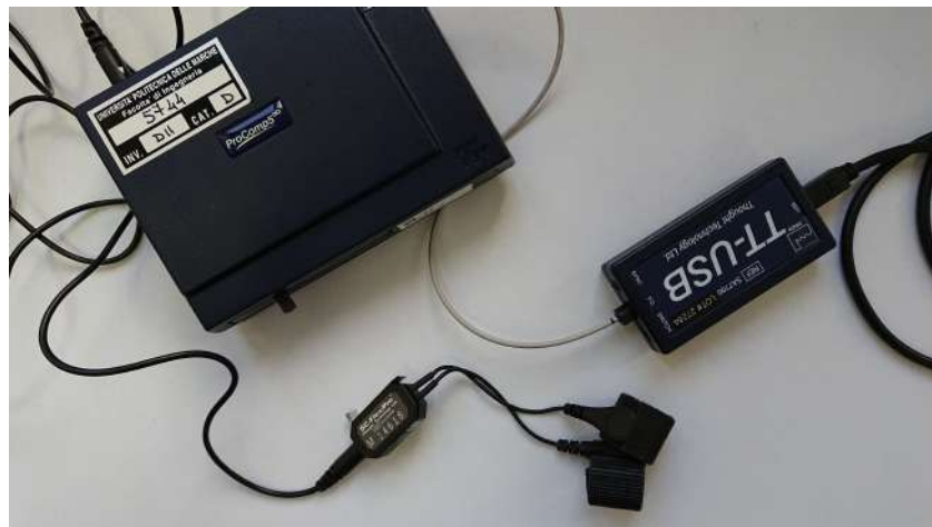
Figure 2. The ProComp Infiniti physiological signals DAQ. The TT-USB hardware interface and the SC sensor are shown.
