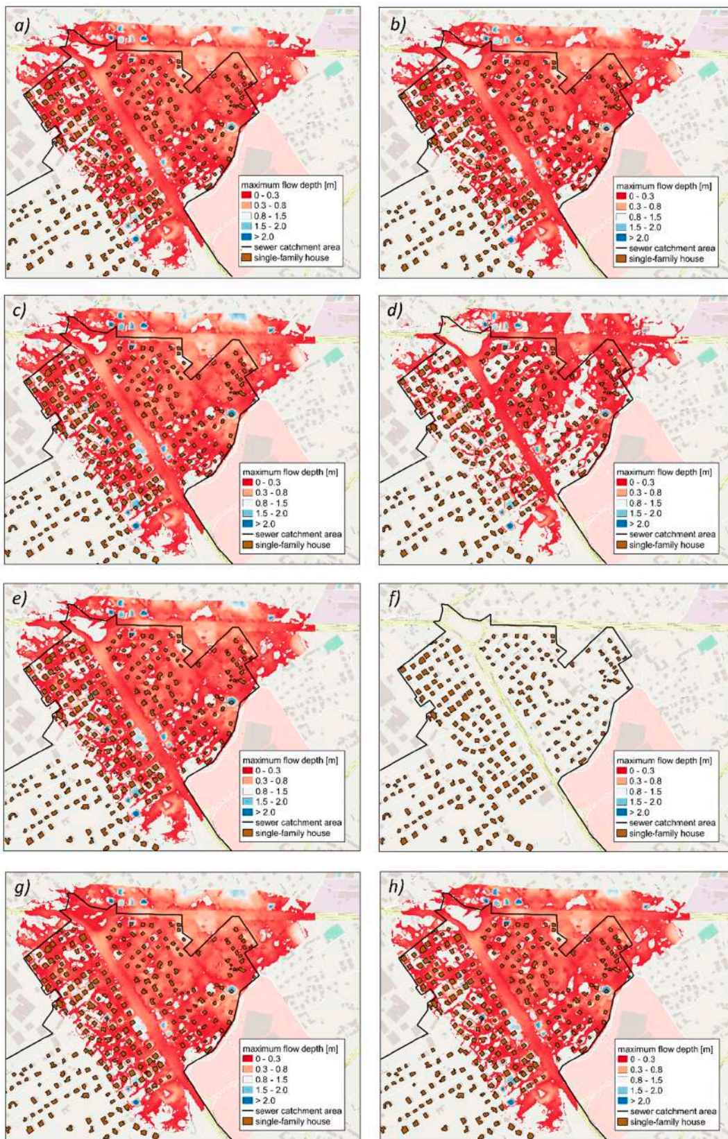
Figure 6. Maximum flow depth for different rainfall events: maximum rainfall event (13 December 2005), (a) no RWH tanks, (b) RWH tanks; average maximum rainfall event (26 September 2003), (c) no RWH tanks, (d) RWH tanks; average rainfall event that produces flood (19 December 2003), (e) no RWH tanks, (f) RWH tanks; the critical event for d = 24 h and T = 5 years, (g) no RWH tanks, (h) RWH tanks.
