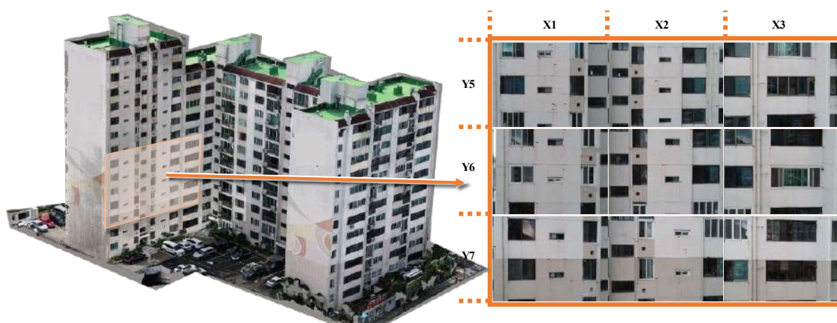
Figure 9. Defect information through 3D modeling and the index method.
