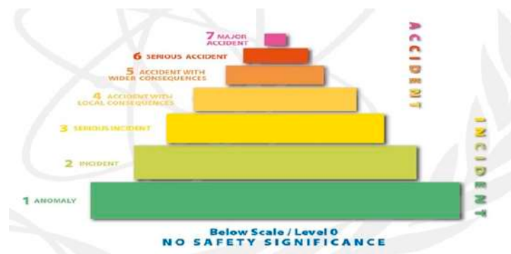
Figure 1. International Nuclear and Radiological Event (INES) Scale. Source: International Atomic Energy Agency official website— https://www-news.iaea.org/InesScale.aspx (accessed on 5 May 2022).
