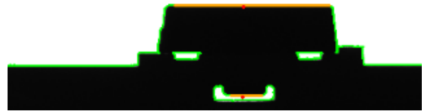
Fig. 9: An image of distance measurement using back-light on object 1
