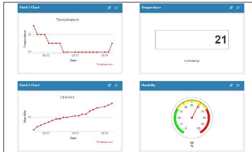
Figure 30. Temperature and humidity from DHT sensor results at the server.
