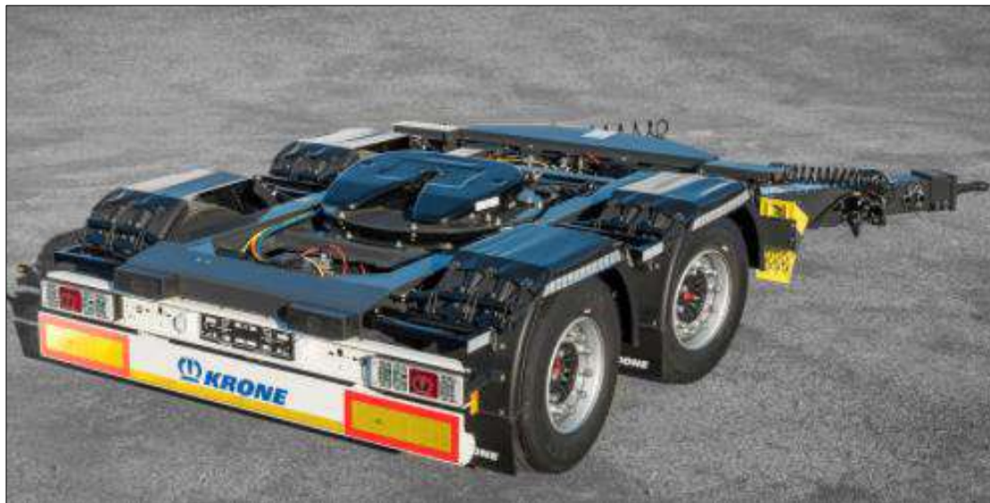
Figure 3. A two axles dolly (Krone, 2017 [5]).
