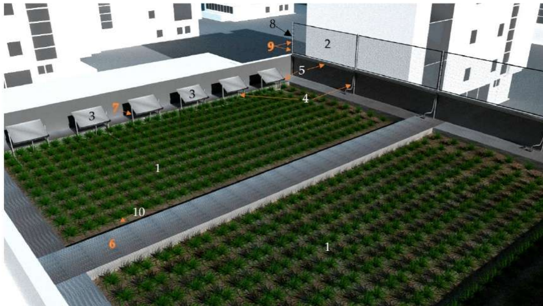
Figure 2. The new design of the green roof with atmospheric water harvesting systems. 1—green roof plants, 2—mesh for fog harvesting, 3—dew collector plate, 4—collector pipe, 5—harvested water collector duct, 6—duct for pipes, 7—metal base for fixing dew collector plate, 8—metal base for mesh installation, 9—metal clamp to fix the mesh, 10—soil.
