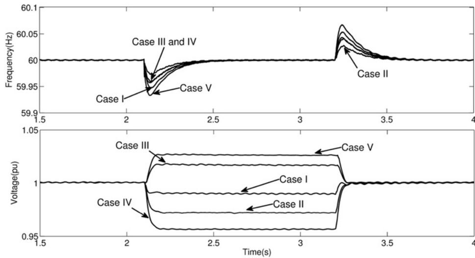
Fig. 7 Frequency and voltage variations during load switching
