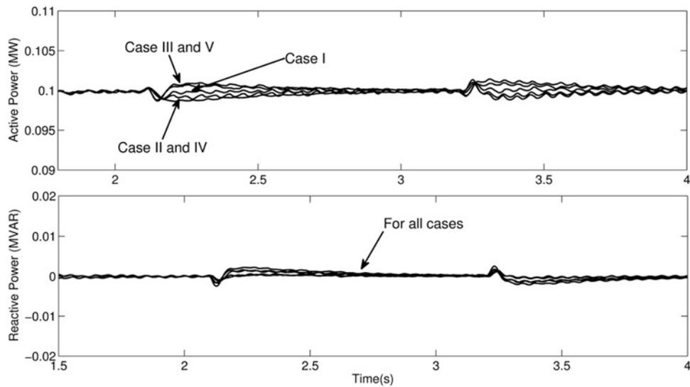
Fig. 8 Active and reactive power variations during load switching
