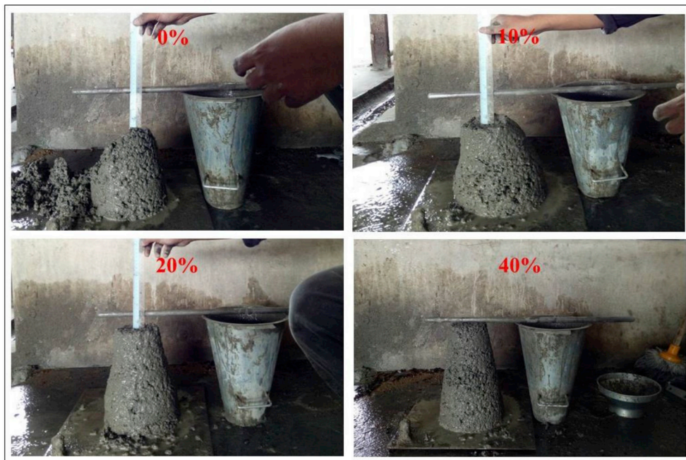
Fig. 6. Workability of OPS lightweight aggregate concrete mixes.
