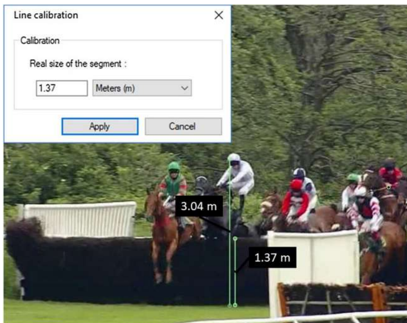
Fig. 3. Example of measurement for jockey head height using a line calibration in horse racing where the height of the fence is known and is taken as the vertical reference height.
