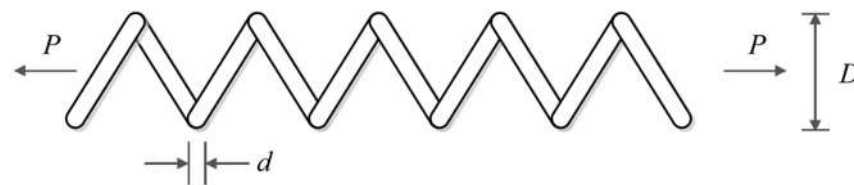
Figure 14. Schematic of tension/compression spring design.
