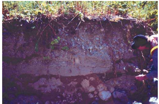
Fig. 4 A profile of sediments on an alluvial (flood) fan showing well sorted layering
