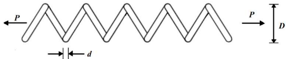
Figure 14. Schematic of the tension/compression spring design.
