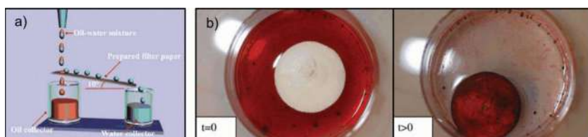
Figure 21. Separation of liquids that differ in surface tension. (a) Illustration of filtration of oil from water through superhydrophobic filter paper (Reproduced with permission. [75] Copyright 2010, American Chemical Society) and (b) absorption of colored hexadecane from water surface by highly porous superhydrophobic nanocellulose aerogel (Reproduced with permission. [93] Copyright 2011, Springer).
