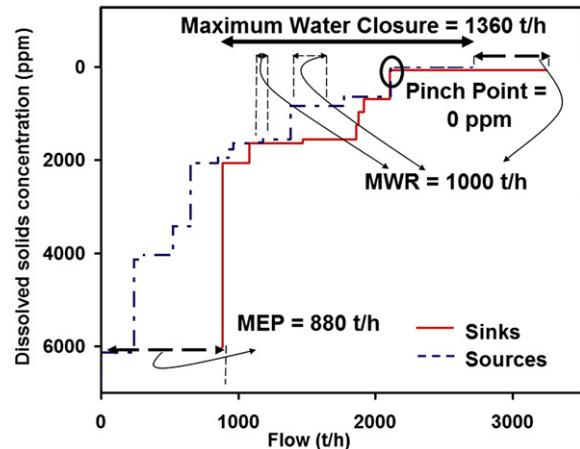
Fig. 6. Water composite curves of the process.
