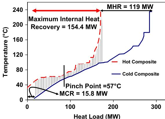
**Fig. 11.** Thermal composite taking into account the elimination of NIM points (HEN-3).
