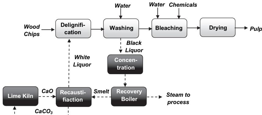
**Fig. 1.** Simplified diagram of the Kraft process.
