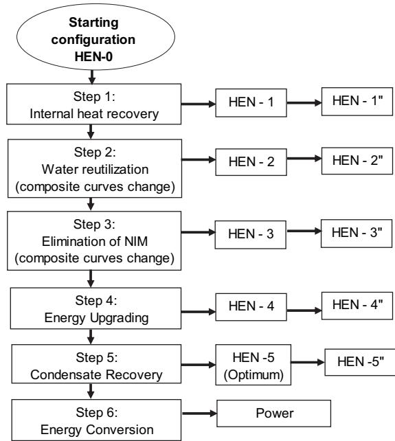
**Fig. 8.** Interactions identification sequential approach.
