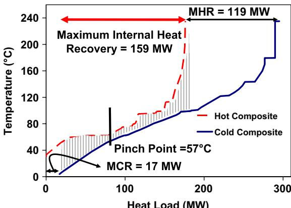
Fig. 5. Thermal composite curves of the process after water reutilization.
