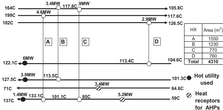
**Fig. 13.** HEN-4: network design above the pinch [36].
