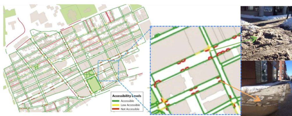
Figure 6. The accessibility condition of the curb cuts in the study area.
