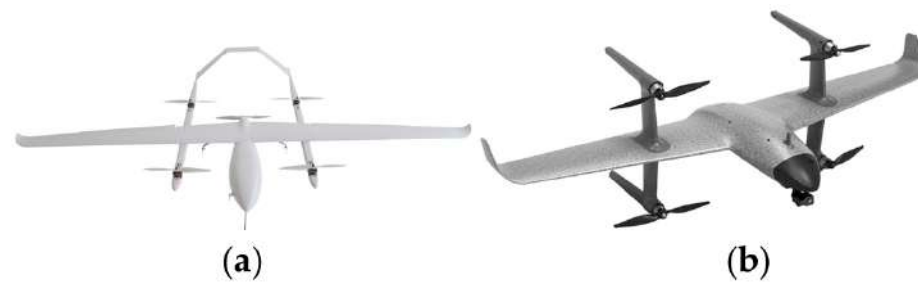
Figure 4. Examples of hybrid UAVs: (a) tilt-rotor aircraft and (b) tilt-wing aircraft.
