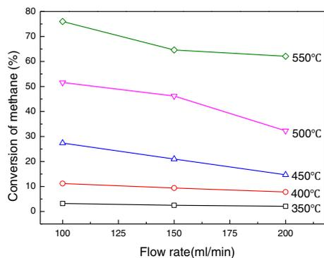
**Figure 4.** Influences of flowrate of the CH<sub>4</sub>-air mixture on the conversion of metal foam I at different temperatures (CH<sub>4</sub> concentration is 5%)
