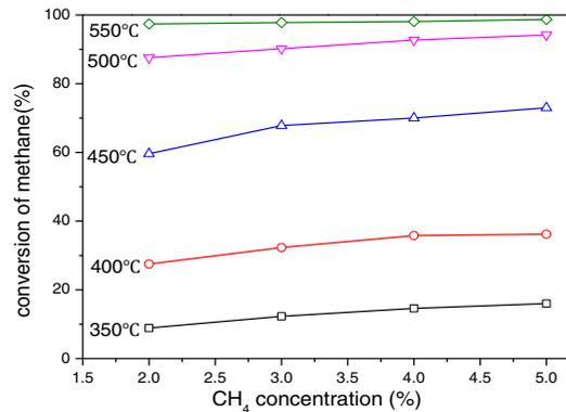
Figure 3. Influences of CH<sub>4</sub> concentration on the activity of the metal foam I (the flow rate of CH<sub>4</sub>-air mixture was set at 50ml/min)
